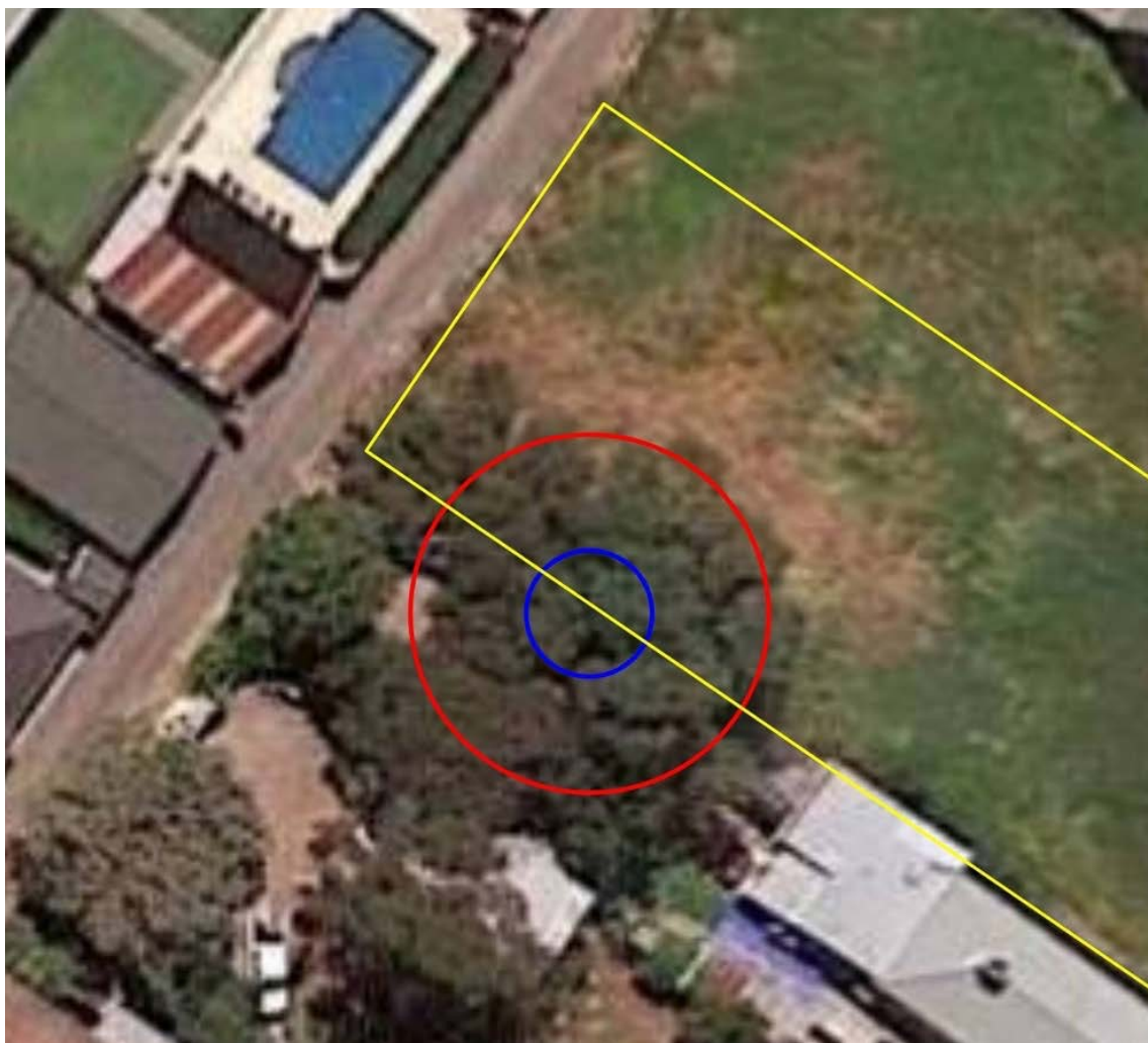
Figure 5: TPZ Plan-existing site.
