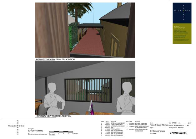
Views showing design of screening to enable views down the driveway to the street whilst precluding southerly views and light spill into adjacent property.
